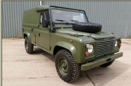
Land Rover Tithonus 110 Defender Hard Top. Fitted 2.5ltr NAD engine, 5 speed gear forward and one reverse gear box, Hi/Low transfer box, Centre Diff lock, Front disc brakes, Rear drum brakes, etc, mileage from 22,000 kms. Excellent condition, Guide Price for RHD £5,000 to £7500 . Guide Price for LHD £6,500 to £8,500 (20 Available)
