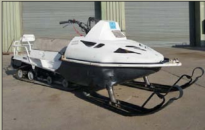
GLX 5900 Ski-doo. Fitted 500cc Rotax Engine, Electric start, 2 forward gears, one hirange, one low range, Reverse gear, Under Seat Stowage compartment, Foot rests Very good Condition, Mileage from 400, Year 2000. Guide Price From £1500 to £3,000 (20 Available) Also Available Pulk Trailer, Guide Price From £350
