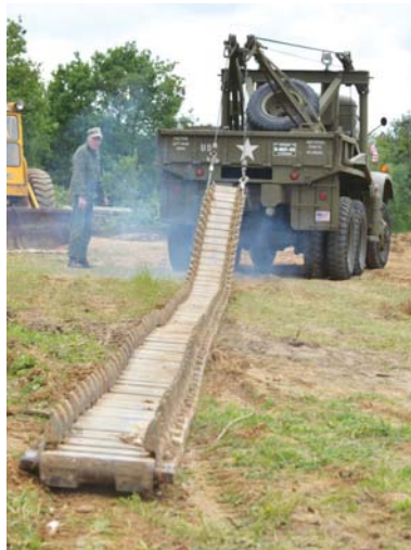
Below right: a Diamond T 969A wrecker uses its Holmes twin booms to drag the broken track away from the tank during the track replacement demonstration.
